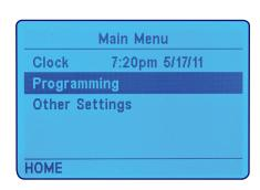
3. Press ⊗ or ⊗ to highlight **Heating Program** or **Cooling Program**, then press **③** (Action button).
