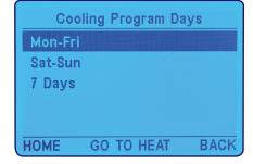
**NOTE:** If the **EXIT** key is pressed at any point while in the Time of Day (TOD) programming menu, the thermostat will return to the previous menu. If any changes are made to a TOD time period or setpoint, the **EXIT** key label will change to **SAVE**.
