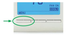
2. Press ⊗ or ⊗ to highlight the **Programming** menu item. Then press ⊚ (Action button) to enter the Programming Menu.
